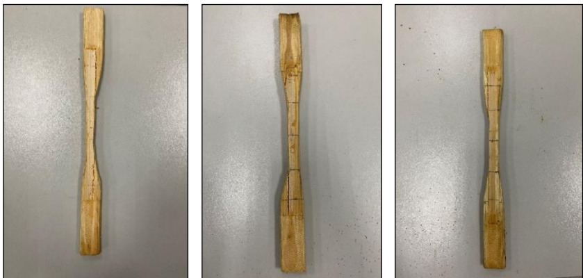
Figure 6. Mode of Failure Tensile Specimen
