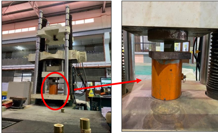
Figure3. Illustrates The Setup for Conducting The Compressive Strength Test
